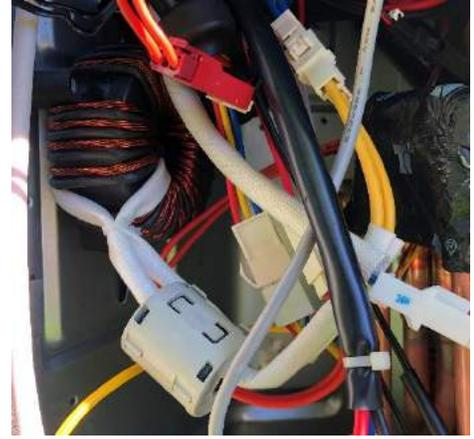
Two checks should be done when testing a Reactor. The first step for both tests is to isolate the reactor, either by removing the wires directly from the Reactor or separating the wire harness if available.
