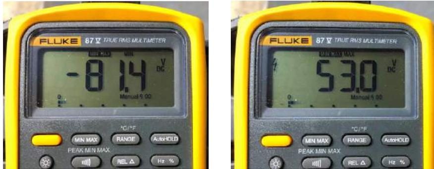
If your meter has a MIN/MAX setting, we recommend using this. It can quickly show you the top and bottom of the alternating range.
