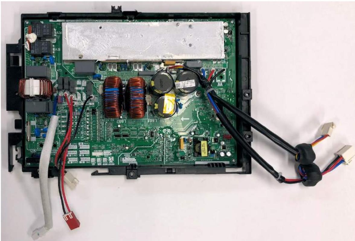
Some wires will be reused when replacing PCB.
