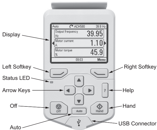
Fig. 57 — ACH580 VFD Keypad — Front
